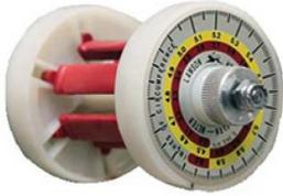
**PRECISE YARN LENGTH** is achieved by Yarn Meter Head, which is a calibrated, adjustable positive yarn feed mechanism that is geared directly to the knitting cylinder. This device ensures that the same amount of yarn is let off for every single cylinder revolution.
