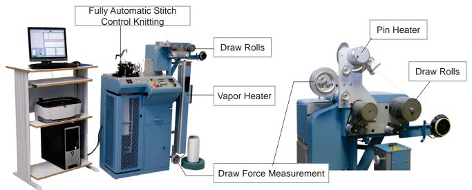
HDK Lab Knitter with Drawing System Main Components
